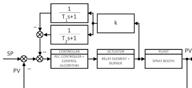
Fig. 5. A two state PID control algorithm
