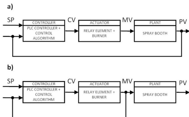
Fig. 4. Structures of a feedback loop, where : a) - a typical structure (the temperature marked as a TT3 is taken as a feedback value); b) a modified structure (the temperature marked as a TT2 is taken as a feedback value)
