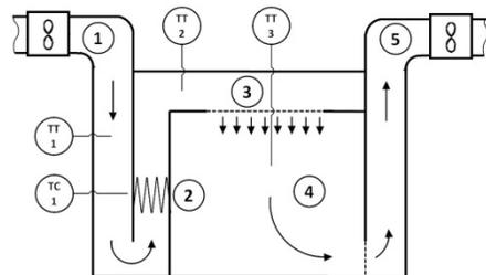
Fig. 1. A PI&D diagram of the spray booth temperature control system
