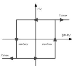
Fig. 3. A static characteristic of the two state control algorithm, where:  $CV_{max}$  - an amplitude of the control signal for ON state,  $CV_{min}$  - an amplitude of the control signal for OFF state,  $minError$ ,  $maxError$  - the minimum value of error for a switch on operation and a maximum value of error for a switch off operation, respectively. In practise it is usually:  $minError = -maxError$
