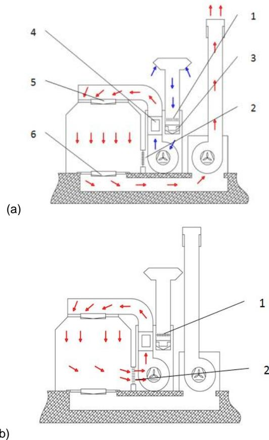
Fig. 1. Typical spray booth in painting mode (a) and drying mode (b), 1 – damper of the suction duct, 2- recirculation damper, 3 – preliminary filter, 4 – burner, 5 – ceiling filter, 6- paint stop filter.
