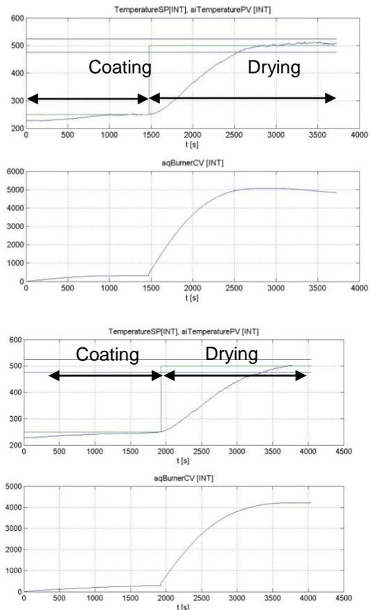
Fig.4. Selected results of the temperature stabilization with the PID control algorithm type ISA.
