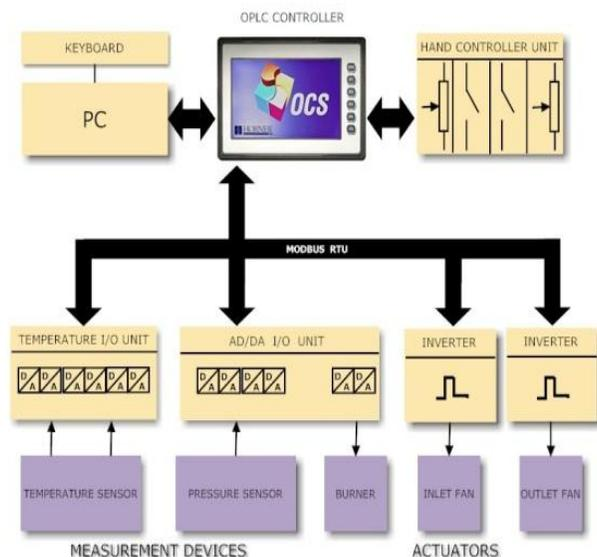
Fig. 3 A general diagram of the spray booth' digital control system.
